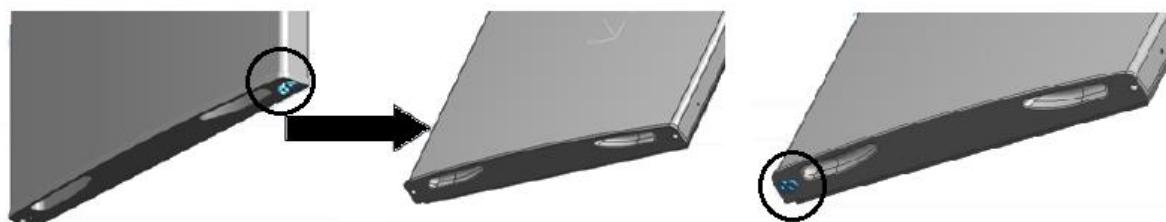
4. Unscrew the screws of the bottom hinge (flat-head screwdriver).
