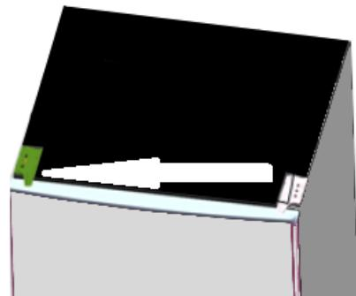
10. Insert the top door and fix the top hinge and top hinge cover.
