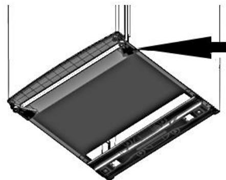
5. Install the door blockers and bearing-bush.
