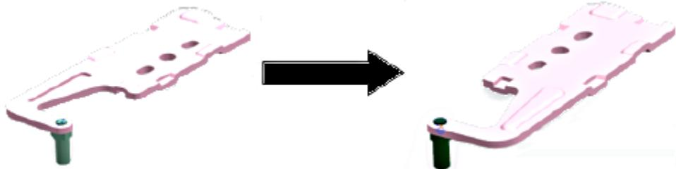
B. Remove the door blockers (top and bottom).
