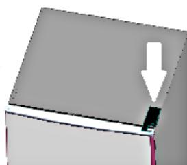
2. Unscrew the screws of the top hinge (flat-head screwdriver).
